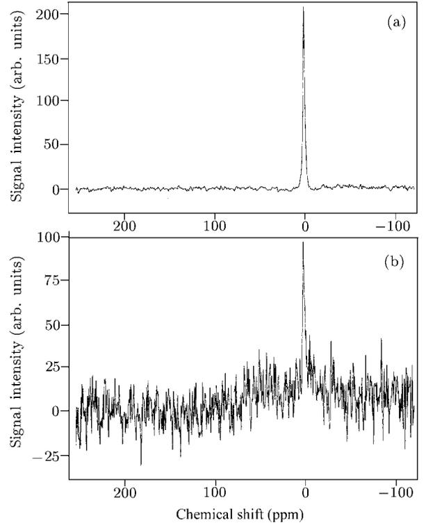
**Fig. 1.** (a) NMR signal of the hyperpolarized  $^{129}\text{Xe}$  produced by spin-exchange with optically pumped  $^{133}\text{Cs}$  in a flow system at 200 K with one scan. (b) NMR signal of the thermally polarized  $^{129}\text{Xe}$  without optical pumping in a flow system at 200 K with 5000 scans.
