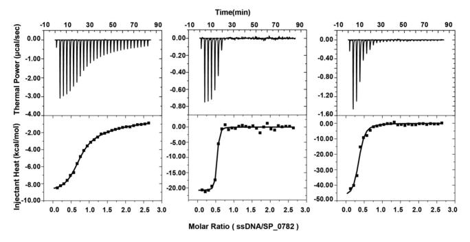
Figure 3. Interactions between SP\_0782 and different lengths of ssDNA (dT6, dT12 and dT19G1) studied by ITC experiments. (Top) Thermal power versus time as indicated. (Bottom) Injection heat versus ssDNA:SP\_0782 (monomer) molar ratio. The resulting parameters, such as stoichiometric ratio (N) and dissociation constant  $(K_D)$ , are indicated in Table 1.
